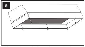
Reinstall the main liner plate to the base of the custom hood and secure it with (5) 3/4" screws.
